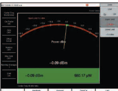
High Accuracy Power Meter provides true RMS measurements from -30 dBm to +20 dBm.
