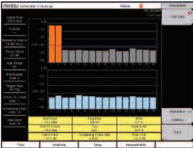
Code Domain Power of the Data Codes is displayed as a bar graph along with the Code Domain Error.
