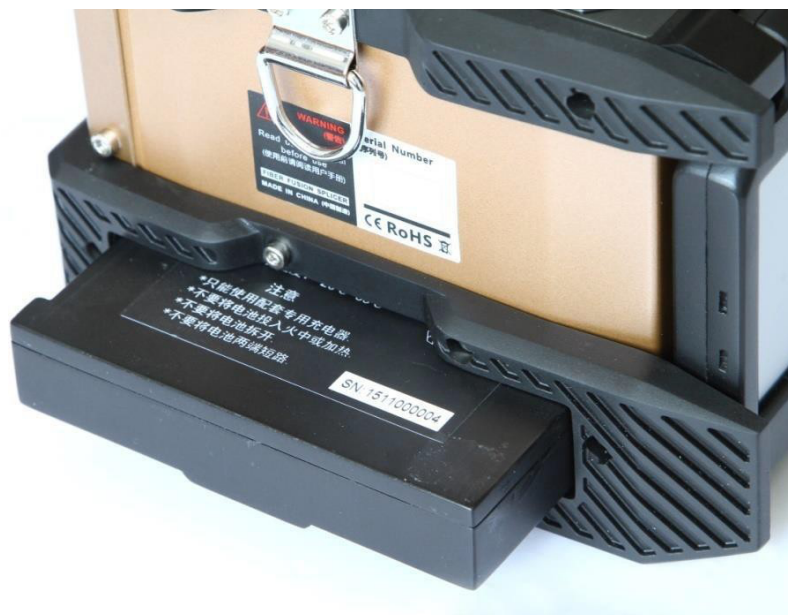
Built-in pluggable lithium battery with large-capacity
